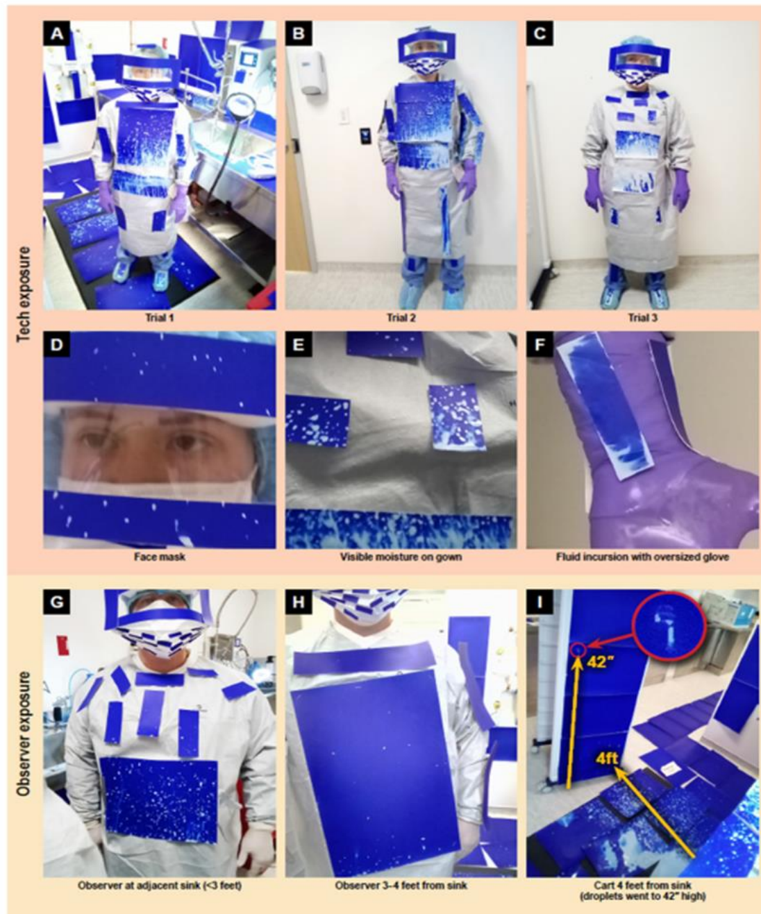
Fig 3. PPE exposure to droplets generated during probe decontamination activities.
